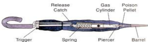
Fig 2. Umbrella gun with which Mr. Georgi Markov was attacked
