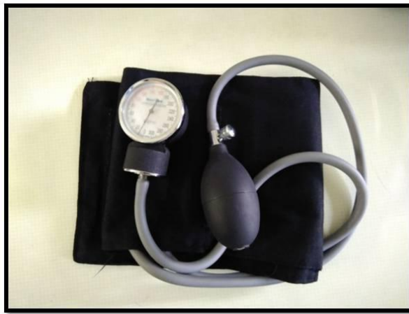
Fig 1. Sphygmomanometer (aneroid manometer)
